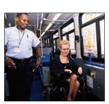
The wheelchair securement area is near the front of the bus. Wheelchairs and mobility devices are secured by tie downs. There is a lap belt for safety.
