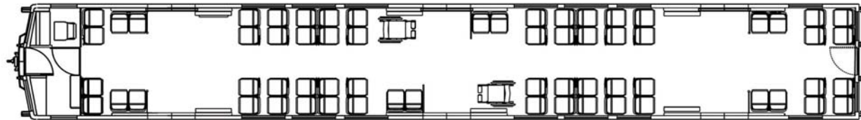
7000 INTERIOR FLOOR PLAN A-CAR
